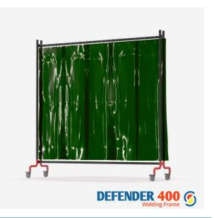
Our top of the range screen. Heavy duty castor wheels, 2 of which are lockable, allowing full mobility. Included with the kit is a pack of EN1598 welding strips, available in red or green. These consist of 5 strips that fasten together by click studs to its neighbouring strip, before attaching via curtain rings to the header rail.
