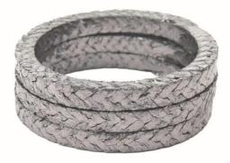
chemical resistance and is suitable for use in applications involving a wide range of media (with the exception of strong oxidising chemicals). This packing material is particularly suitable for sealing high pressure, high temperature valves in oil & gas, petrochemical and general industries.
