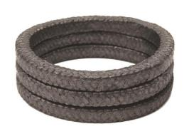
yarn reinforcement provides stability, resilience and anti-extrusion properties. This packing style does not damage / wear the shaft / spindle. Typical sealing applications include use in power generation (steam valves, boiler-feed pumps, condensate pumps etc), chemical and petrochemical industries. Suitable for most chemicals except strong oxidizing agents such as sulphuric and nitric acids in high concentrations, oleum and aqua-regia.
