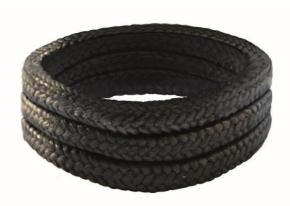
Materials of construction: Continuous filament Glass yarn's impregnated with PTFE dispersion and lubricated with mineral oil and graphite.
